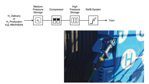
A typical compressed hydrogen road tank holds around 1,100 kg of fuel; liquid storage tanks hold around 3,500kg. Over 600 km the iLINT train in German was estimated to consume around 138 kg of hydrogen. This increases to 2,000 kg per day for 14 trains.
