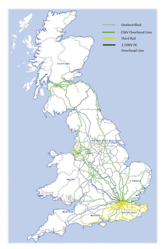
Figure 4: UK Rail network showing 25kV electrification in green and 750V DC third rail in yellow
