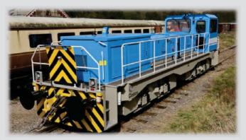
Using lead-acid battery technology with on board hybrid batter charging these shunting locomotives can offer long-range haulage at relatively low speeds with zero-emissions. As well as this they operate at low noise levels and provide opportunities for operational and maintenance cost savings.
