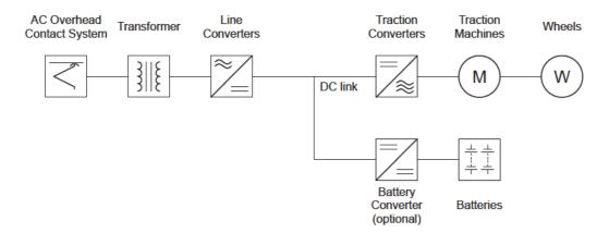
The performance characteristics of battery powered trains are limited in some areas, such as range and top speed. Although it is possible to continue to fit more and more batteries to increase performance, the economic benefit diminishes as the weight of on-board batteries and control systems increases relative to the capacity of the train. The market conditions on the continent in 2019 suggest the following performance characteristics:
