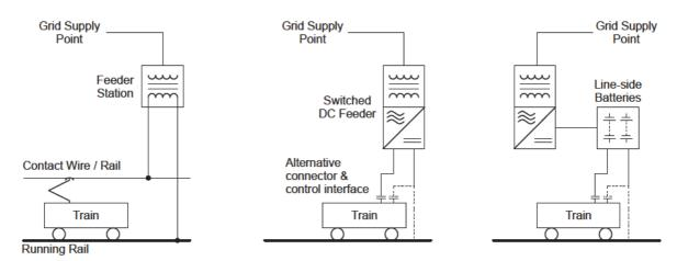
The static charging facility needs a connection to the National Grid. The size of the supply needed will depend on the charging power required and the amount of trains being charged at any one time. Likely static charge power can range from hundreds of kilo Watts to several Mega Watts; therefore, dedicated grid connections can be smaller than those for continuous contact systems.
