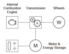
Hybridisation involves the addition of energy storage and conversion equipment, so is typically expected to increase the weight of a multiple unit vehicle depending on design. The main advantages are an expected fuel saving of around 20%, although this is heavily influenced by the driving cycle.
